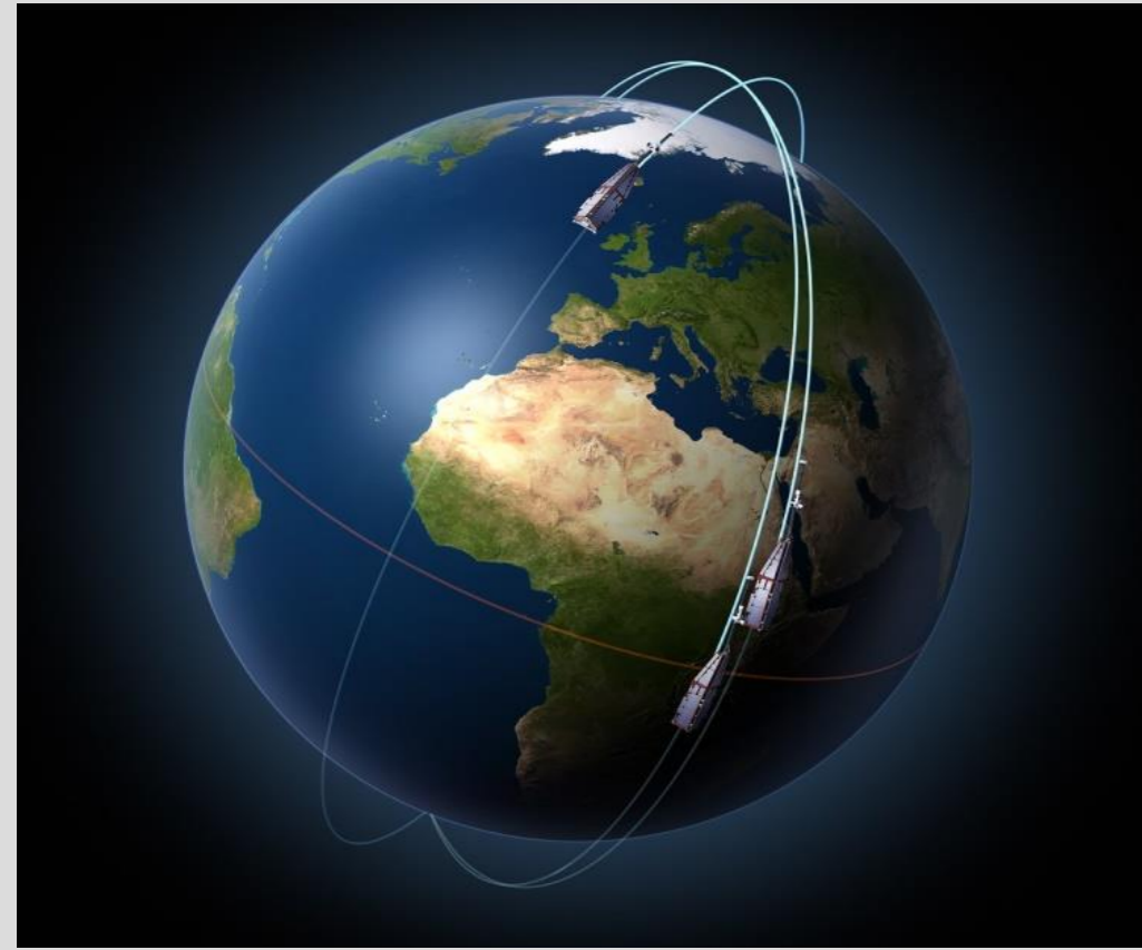
Figure 1: Artist's view of Swarm constellation (left, ©ESA/ATG Media lab): Two satellites are flying in pendulum formation at near-polar orbits with an initial altitude of 460 km, the third flying in a higher 530 km orbit. Absolute and relative orbit determination can be done using the onboard GPS system (right).
